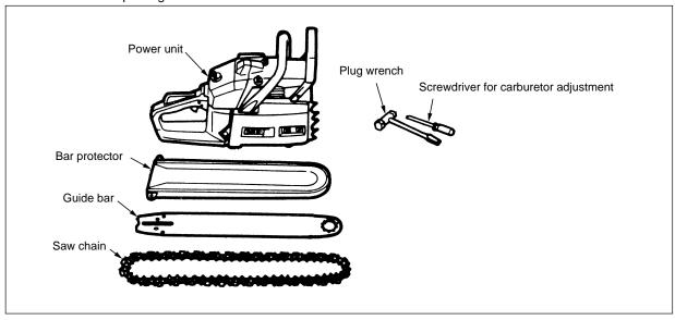
Open the box and install the guide bar and the saw chain on the power unit as follows:
